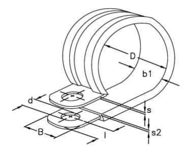
$\begin{array}{lll} b1 & = 15.0 \\ d & = 6.4 \\ Diameter D = 40 \\ I & = 6 \\ s & = 0.8 \\ s2 & = 1.2 \\ Width B & = 12 \\ \end{array}$
